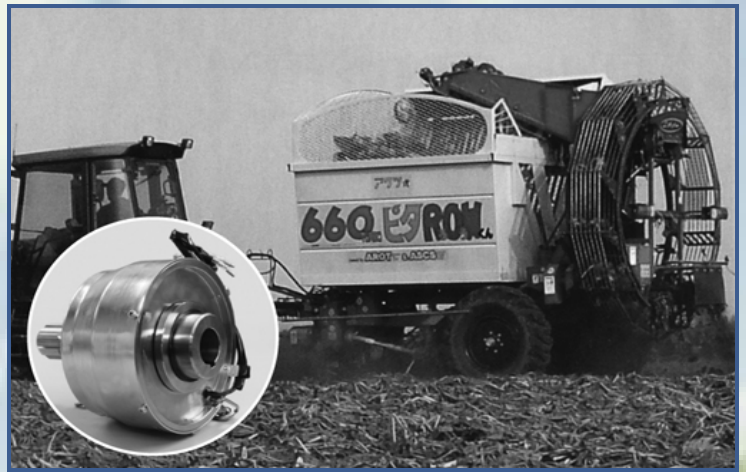
Beet Harvester with SMC Spring Applied Clutch
